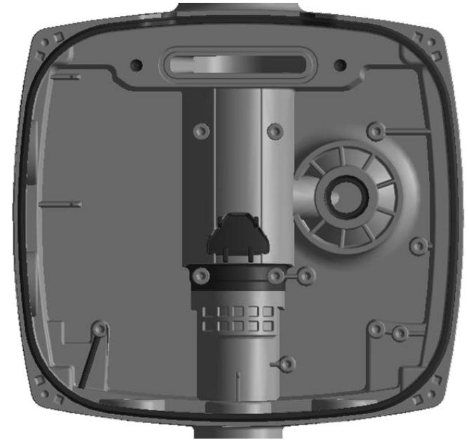
New seat for the pressure sensor
